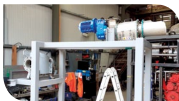
Macerator & Separator in mobile framework, for placement in Trailer 1
