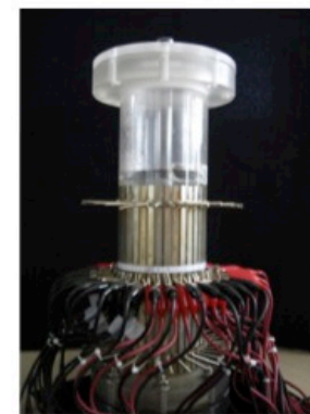
Phantom with boundary electrodes where electric current is injected and voltages are recorded
