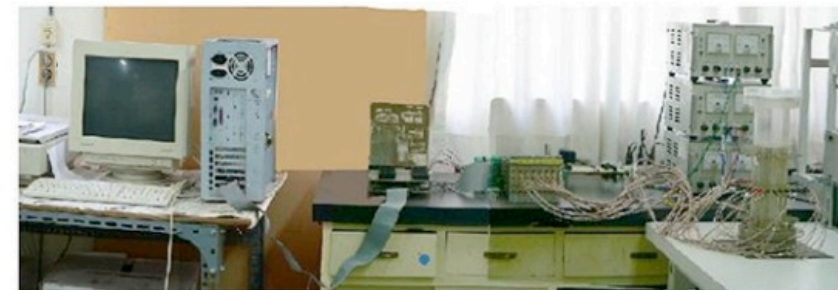
Dynamic Electrical Impedance Tomography Measurement System
