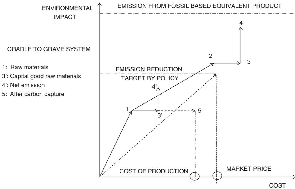
Figure 5.17 Added cost and environmental impact (contribution analysis) of biorefinery cradle to grave systems.
