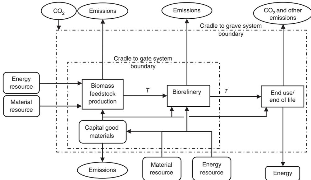
**Figure 5.15** A biorefinery system has biomass production, product manufacturing, end use and construction materials' life cycle process blocks. *T* shows where the transportation of materials is involved.
