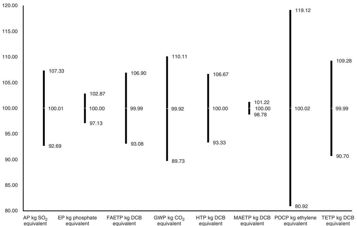
**Figure 5.5** Sewage sludge to micro generation and digested matter: range of variations from the mean values due to  $\pm 25\%$  standard deviation in the independent variable (biogas volumetric production rate).
