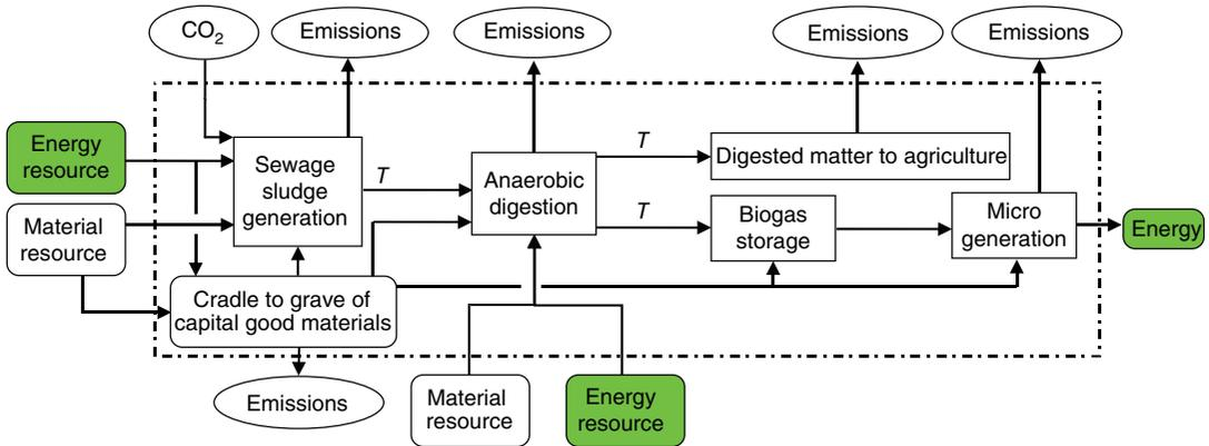
**Figure 5.18** Cradle to grave anaerobic digestion of sewage sludge system for LCA. *T* stands for transport.
