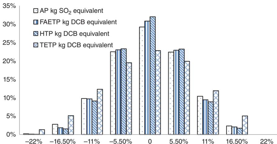
**Figure 5.10** Acidification, freshwater aquatic ecotoxicity, human toxicity and terrestrial ecotoxicity potentials (AP, FAETP, HTP and TETP) impact probability distributions (y axis) with respect to standard deviations (x axis) from their mean values.
