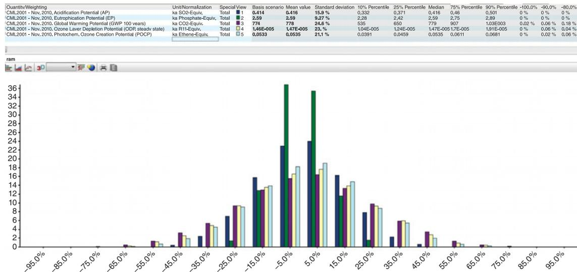
**Figure 5.12** Probability distribution versus standard deviation from the mean value of various impact categories using GaBi software.
