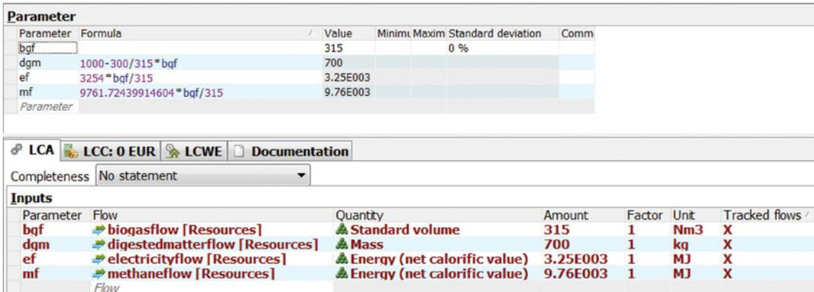
Figure 5.7 Screenshot from GaBi, to define the independent and dependent parameters involved in an AD plant LCA study.
