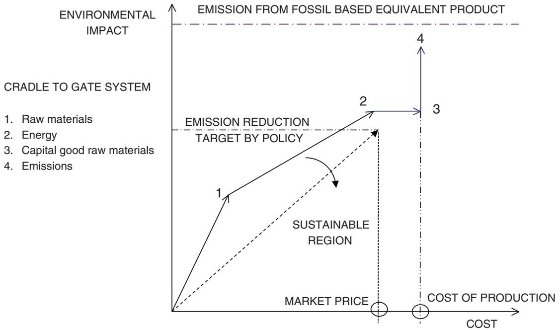
Figure 5.16 Added cost and environmental impact (contribution analysis) of biorefinery cradle to gate systems.
