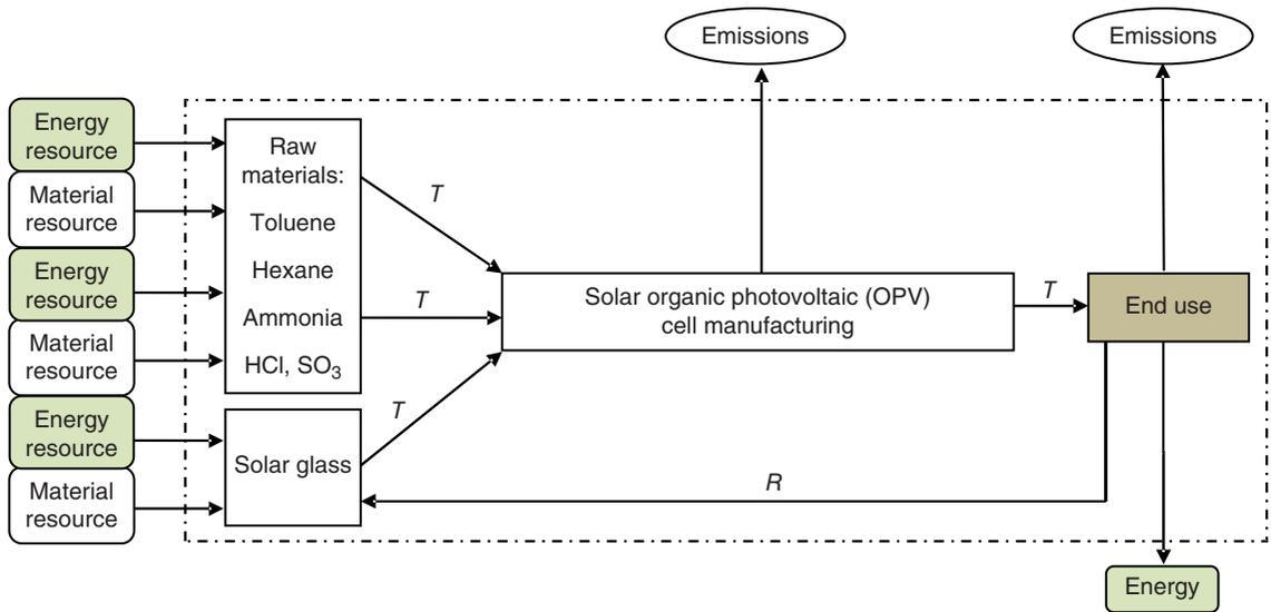
**Figure 5.20** Cradle to grave solar OPV cell manufacturing system for LCA. *T* stands for transport. *R* stands for recycle. *T* and *R* also cause resource depletion and environmental emissions. Only a part of “End use” block impacts due to solar cell manufacturing needs to be considered within the system boundary.
