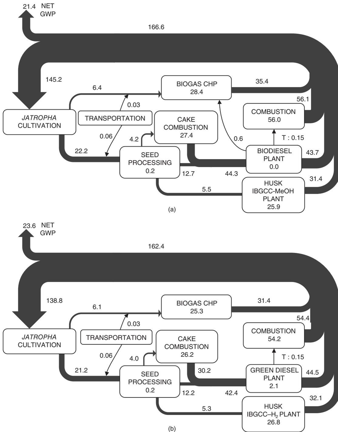
**Figure 5.2** Sankey diagram for GWP (as CO<sub>2</sub> equivalent) flows in g MJ<sup>-1</sup> in two integrated whole Jatropa fruit biorefinery systems producing heat and power and (a) biodiesel or (b) green diesel.
