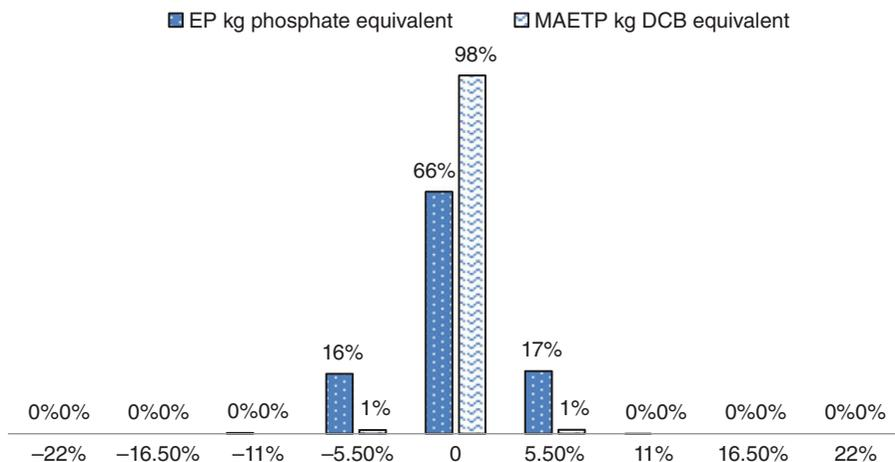
**Figure 5.11** Probability distributions (y axis) of marine aquatic ecotoxicity potential (MAETP) and eutrophication potential (EP) with respect to standard deviations (x axis) from their mean values.
