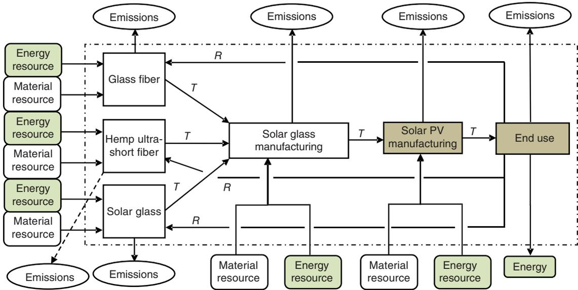
**Figure 5.19** Cradle to grave solar organic photovoltaic (OPV) glass manufacturing system for LCA. *T* stands for transport. *R* stands for recycle. *T* and *R* also cause resource depletion and environmental emissions. Only a part of “Solar PV manufacturing” and “End use” block impacts due to solar glass manufacturing needs to be considered within the system boundary.
