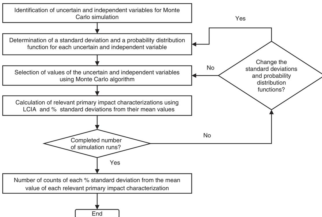
**Figure 5.6** Monte Carlo simulation framework integrated with LCA.
