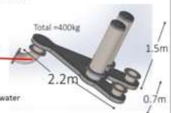
World's largest fluidic oscillator: Throughput ~2400 cubic metres / hr
