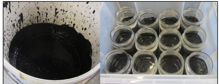
The digestate (left) from wastewater biosolids has a relatively low solids content. Other digestates from food and agro-wastes (right) have higher solids content and different rheological properties which make dewatering more challenging
