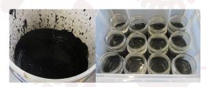
Digestate from wastewater biosolids (left) has a relatively low solids content. Other digestates from food and agro-wastes (right) have higher solids content and different rheological properties which make dewatering more challenging
