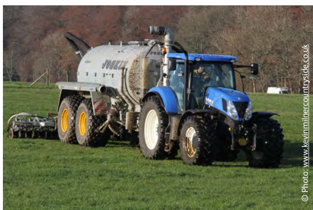
Figure 14: Low emissions slurry injection equipment
