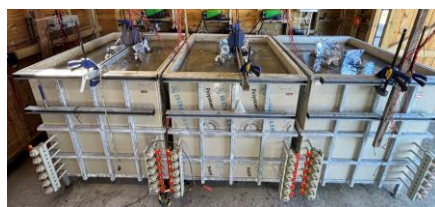
Fig: 1 \text{ m}^3 tank with 4x tubular MEC
